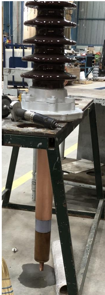
Fig 4 – Visually inspect for damage or oil leaking.
