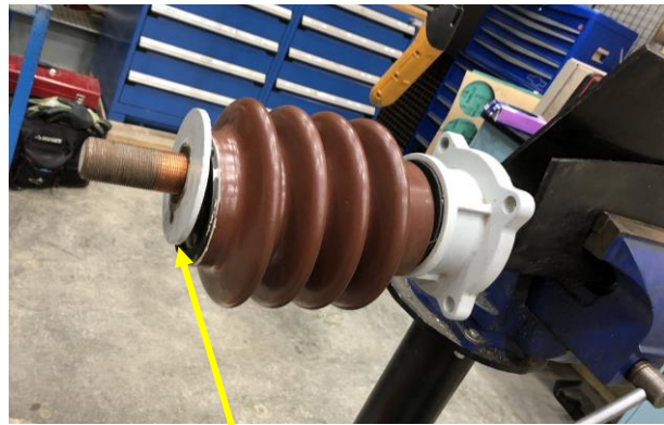
Fig 9 - Bevelled washer
