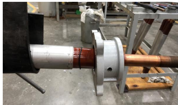
Fig 13 – Removing the flange
