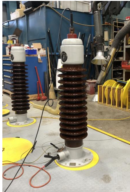
Fig 3 – Bushing testing at the central maintenance services at Hydro One.
