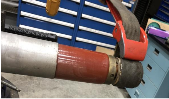
Fig 14 – Removing the bottom connecting end
